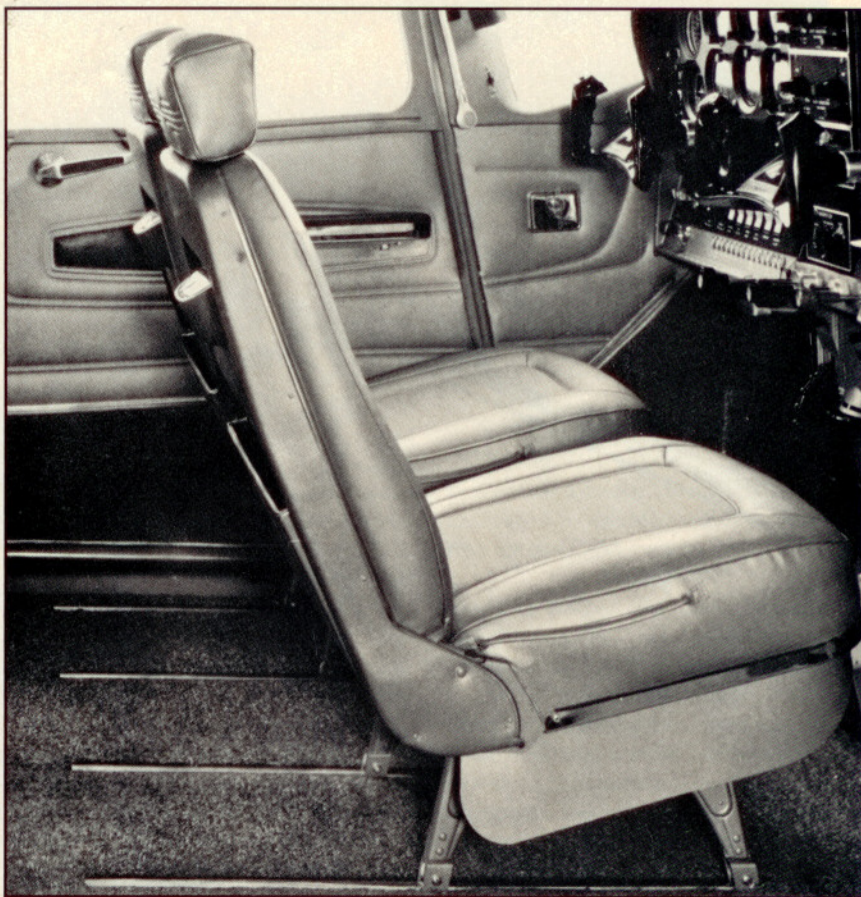
Interior shot of 1969 Skylane shows one reason for seat track wear: seats must slide forward for rear passengers to enter, aft for front occupants.
